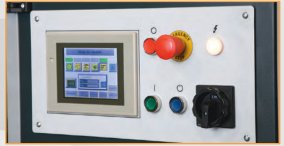
Touch screen control panel for machine functions management
